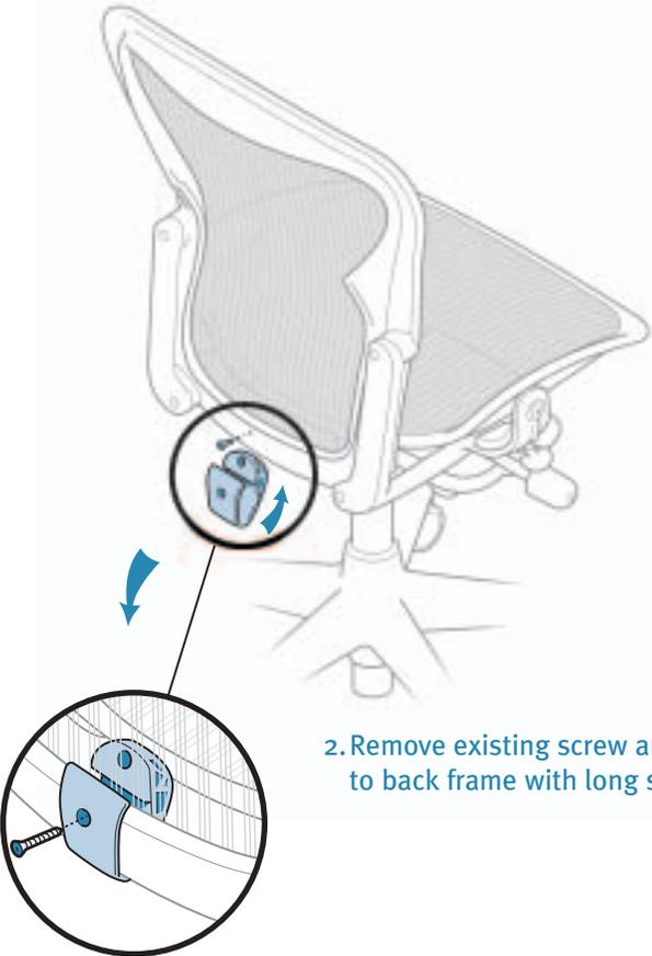
2. Remove existing screw and install clip to back frame with long screw from kit
