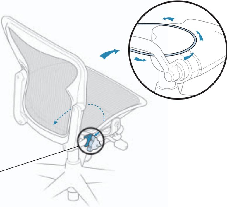
3. Attach control mechanism to right swing arm
