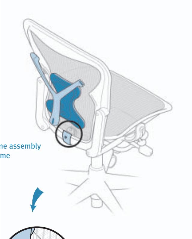
6. Attach cable end to wishbone assembly
